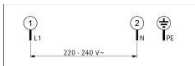
Fig. 4.86 1-phase connection diagram
